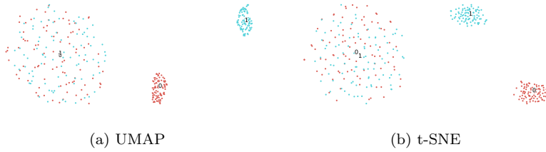
Fig. 19 Projection to two dimensions of ShapeletSim dataset between Raw (left) and DNN’s Latent space (right) with either UMAP or t-SNE. The latent space is obtained with ResNet-multi-rec-None .
